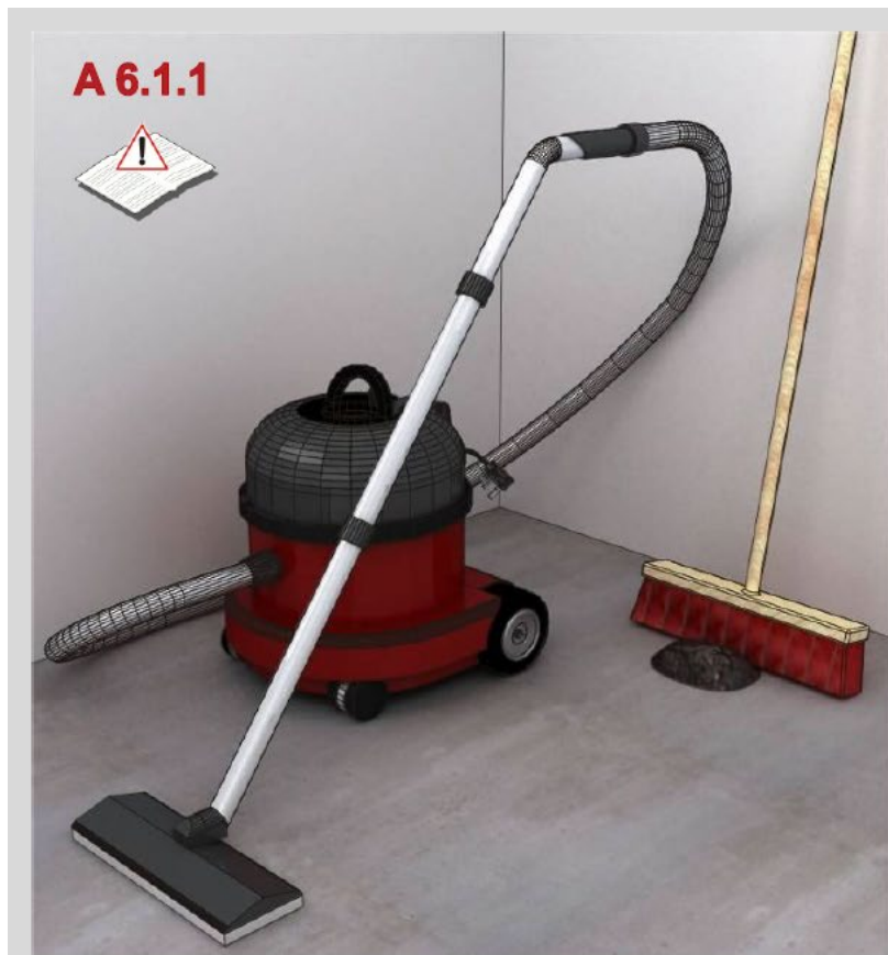
Picture 4 Cleaning of the subfloor
